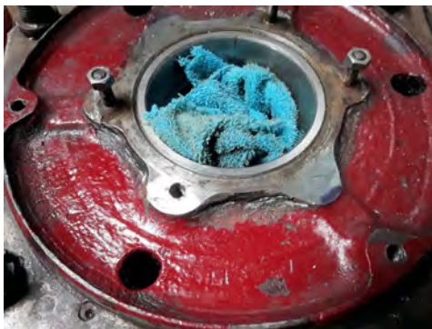
Cardiff 262. The front hub, showing the four studs that require renewing. [Keith Walker]
