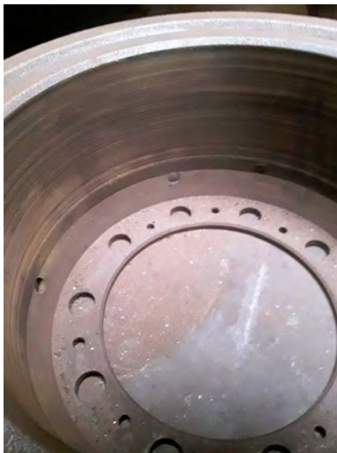
The condition of the inner surface of the brake drums which are offsite for machining. [Keith Walker]
