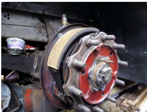
A front pair of newly relined front shoes for 243. [Keith Walker]
